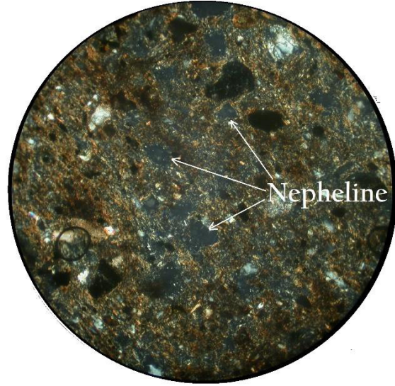
Figure 15: Sample No. 6. X 40 magnification. Light XPL, residue of nepheline (photo by authors).
