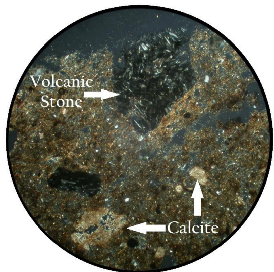
Figure. 18: Sample No. 10. X 40 magnification. XPL Light, porphyry texture, residue of calcite and volcanic stone (photo by authors).
