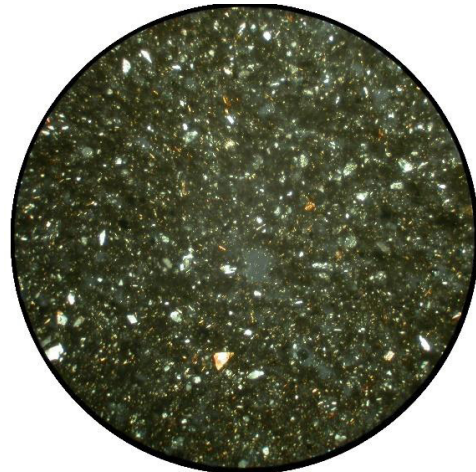
Figure. 9: Sample No. 4, X 40 magnification. Light XPL, silty paste with numerous pieces of small quartz (photo by authors).
